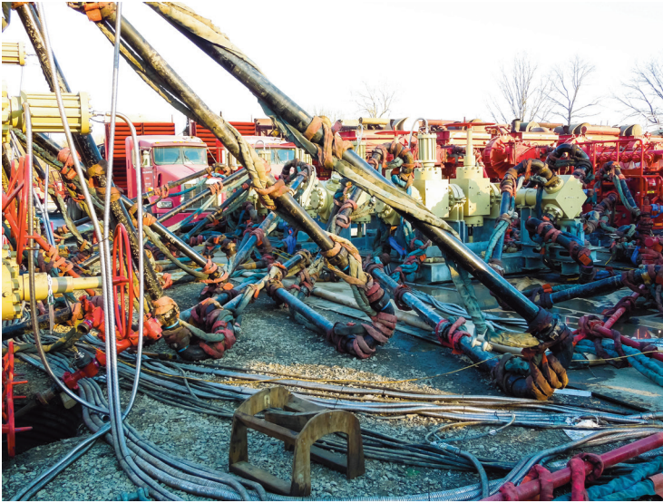
Figure 5. One of the standard responses to these conditions has been to put more fluid through more lines. But, that only adds to an already tangled maze of lines on the well pad.
