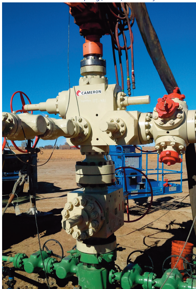
Figure 4. The F-T90 is engineered 50% smaller and 25% lighter than conventional frack trees while preserving the rigorous durability and reliability required by the industry.
