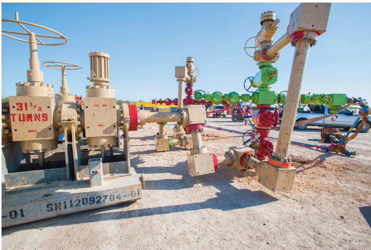
Figure 6. One answer is Cameron's Monoline™ Frac Fluid Delivery System. This system replaces the need to rig-up four separate flow lines to the frack tree with a single line featuring a large inner diameter bore to accommodate the large frack fluid volumes required in today's hydraulic fracturing programmes.
