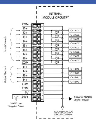
Note: This module includes input and output channels. Before connecting field wiring, verify that you are connecting to the appropriate terminals
