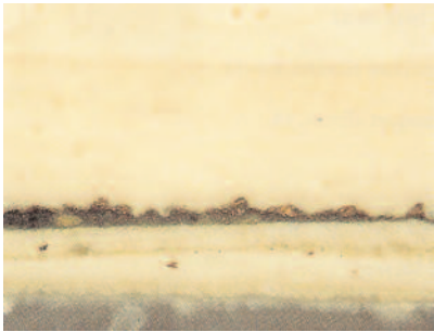
Figure 7 Cross section from an area of bronzing, dating from 1802, on a caryatid in the Breakfast Room at Pitzhanger Manor, Ealing, Middlesex. Viewed by reflected visible light (quartz-halogen source). Above the Coade stone substrate are several layers of white, a coat of dark green, and bronze powder entrapped in a varnish medium.
