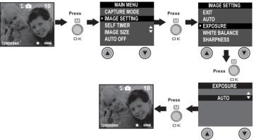
You can adjust the exposure compensation value (EV) within the range of -1.5EV to +1.5EV in order to compensate for current lighting conditions. This setting can be used to obtain better result when shooting with backlighting, indirect indoor lighting, a dark background, etc.
