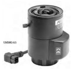
The purpose of Pelco's **13VDIR Series** is to compensate for the focus shift that results from the different wavelengths of visible and IR light. IR corrected lenses focus light energy on the same plane. The result is better focus, sharper contrast, and better overall image quality.
