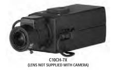
The **C10CH Series** has a standard CS lens mount and can be used with fixed, manual, or auto iris (DC or video drive) lenses. The iris is controlled through a standard 4-pin square connector that is included on all Pelco auto iris lenses.
