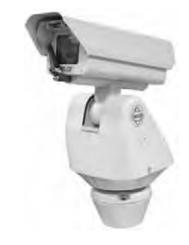
A powder-coated, aluminum construction makes the **ES30PC** and **ES31PC** ideal for either indoor or outdoor applications. The system has an absolute operating temperature range of  $-50^{\circ}$  to  $140^{\circ}$ F (-45° to 50°C). Within two hours after power-up, the entire unit can de-ice and be operational from a temperature of  $-13^{\circ}$ F (-25°C).
