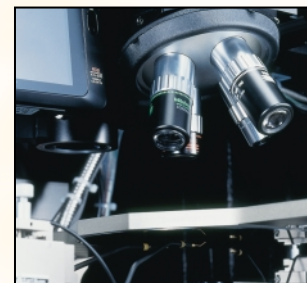
Failure analysis with emission microscopy
