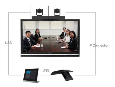
The following figure illustrates the connectivity between EagleEye Director II camera system, Polycom Trio and Surface Hub.
