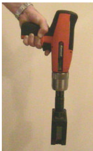
Barrel in extended position. This cocks the tool.
