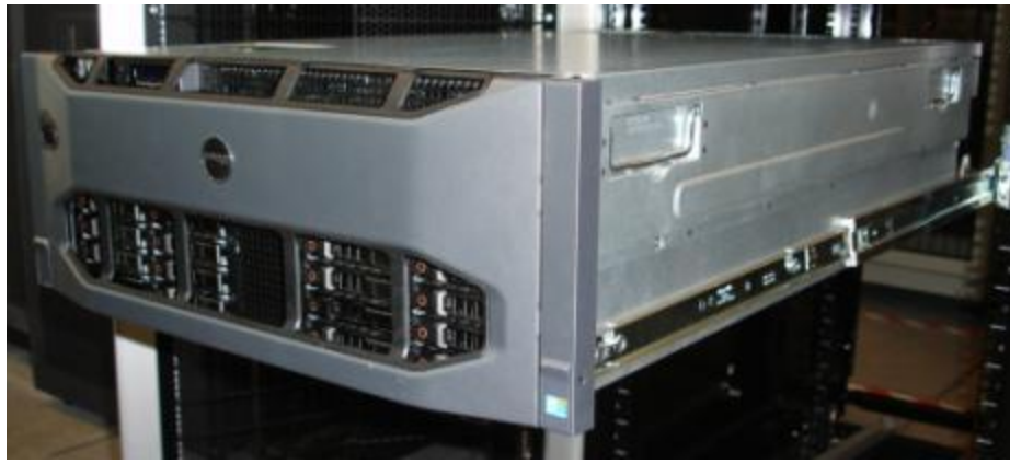
Figure 24. R910 Mounted in the B2 Sliding Rails
