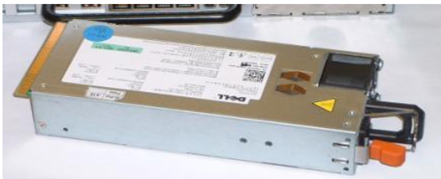
Figure 17. R910 Power Supply
