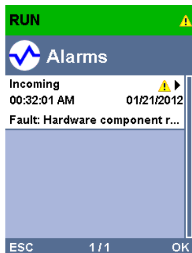
Figure 4-11 Display of alarms
