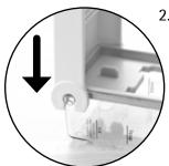
Attach lid to base. Make sure lid is fully seated on hinge before pressing down.
