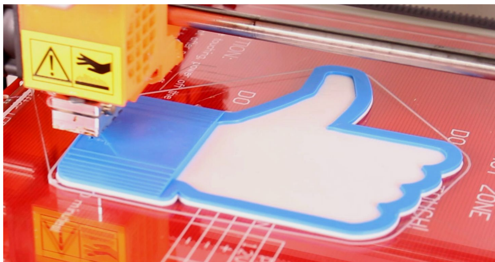
Pict. 21- Multicolored object printed with ColorPrint
