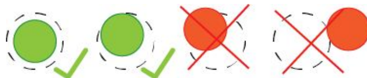
Pic. 6 - The probe must be inside the circles (1st and 9th calibration point) to successfully level the bed.
