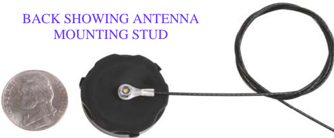
SHOWN WITH LID OFF AND BATTERY REMOVED
