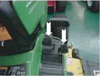
Figure 9. Pedals to operate hydrostatic transmission.
