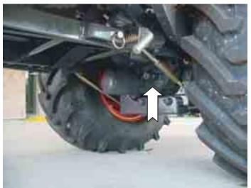
Figure 12. Mid-mount PTO shaft.
