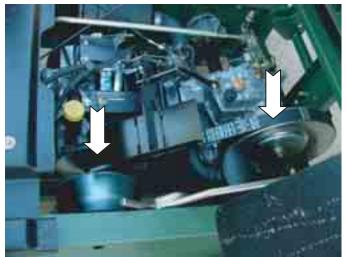
Figure 7. Variable speed belt drive. Arrows point to variable sheaves.
