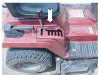
Figure 8. Gearshift lever on gear transmission on lawn tractor.
