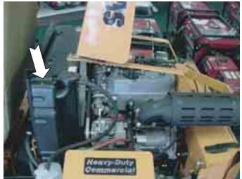
Figure 6. Water-cooled engine arrow points to radiator.
