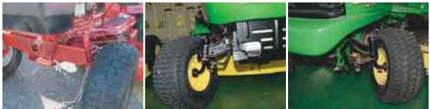
Figure 17. Formed and welded front axle on cheap tractor on the left; cast iron front axle on small lawn tractor in the center, forged front axle on higher quality tractor on the right.
