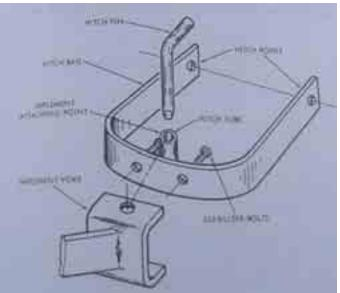
Figure 15. Sleeve hitch: tractor portion on right, implement portion on left.
