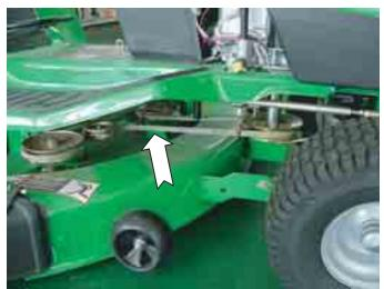
Figure 10. Belt drive to mower deck.
