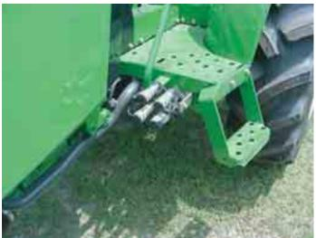
Figure 13. Remote hydraulic outlets on tractor.
