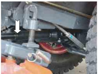
Figure 11. Shaft drive to mower deck.
