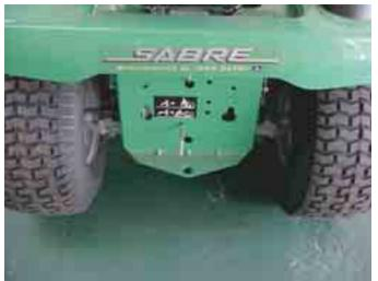
Figure 14. Drawbar hitch on lawn tractor.
