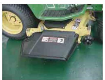
Figure 18. Discharge chute in place.
