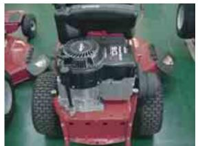
Figure 4. Vertical-shaft engine.
