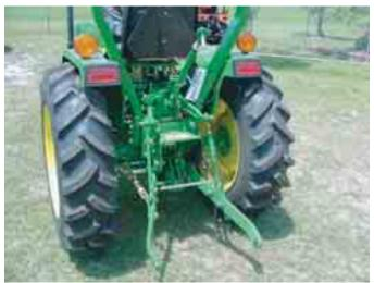
Figure 16. Three point hitch on compact tractor.
