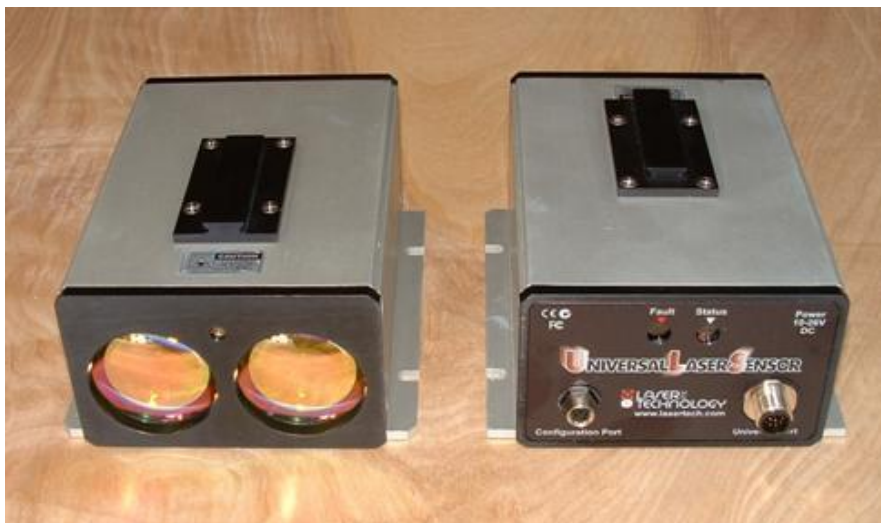
Figure 2-6. Laser Technology infrared Universal Laser Sensors have been used as redundant air gap sensors by NOS/CO-OPS (courtesy of Mark Bushnell, CoastalObsTechServices).
