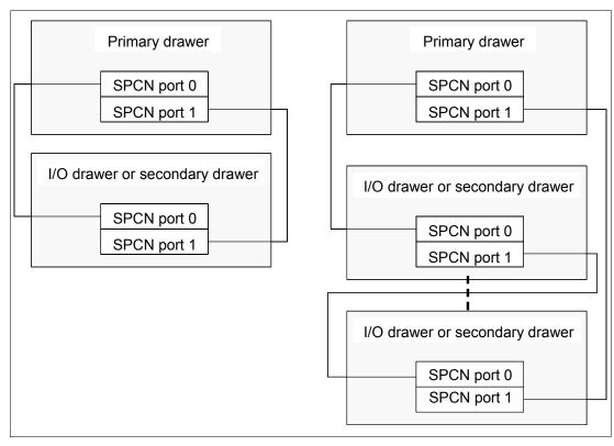
Figure 2-13 SPCN cabling examples
