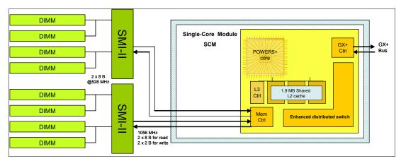
Figure 2-3 p5-520 POWER5+ 1.65 SCM with DDR2 memory socket layout view
