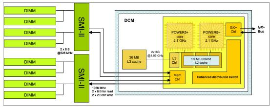
Figure 2-5 The p5-520 POWER5+ 2.1 GHz DCM with DDR2 memory socket layout view
