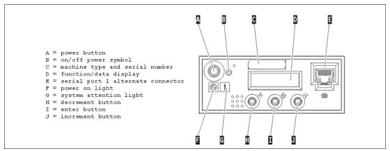
Figure 2-21 Operator control panel physical details and buttons
