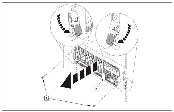
Figure 2-20 Pull the server to the service position
