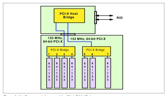
Figure 2-10 Conceptual diagram of the 7311-D20 I/O drawer
