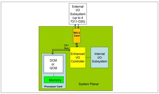
Figure 2-9 p5-520 or p5-520Q GX+ Bus connection overview
