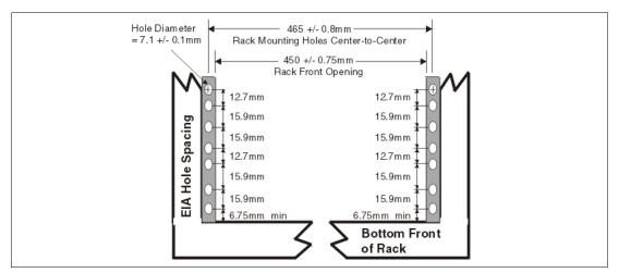
Figure 1-7 Rack specification dimensions, bottom front view
