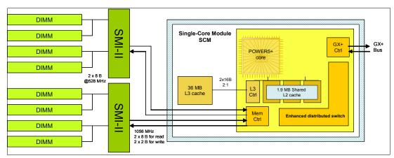
Figure 2-4 p5-520 POWER5+ 2.1 GHz SCM with DDR2 memory socket layout view
