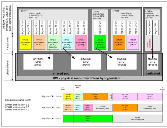
Figure 2-14 Logical, virtual, and physical processor mapping
