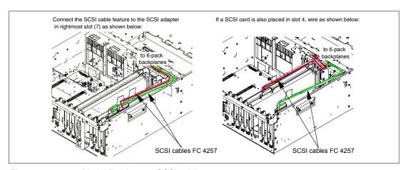
Figure 2-11 7311 Model D20 internal SCSI cabling
