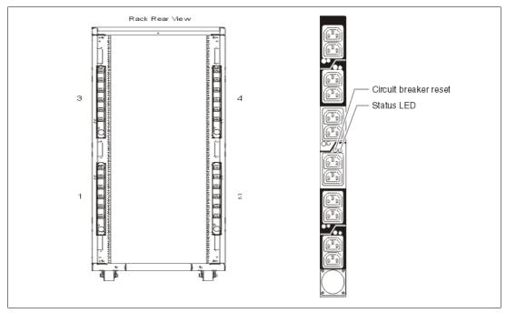
Figure 1-4 PDU placement and PDU view
