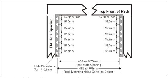
Figure 1-6 Rack specification dimensions, top front view
