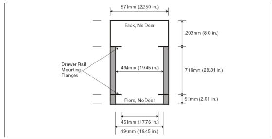
Figure 1-5 Top view of non-IBM rack specification dimensions
