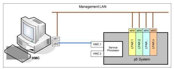
Figure 2-17 HMC to service processor and LPARs network connection
