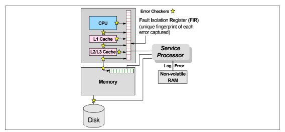
Figure 3-1 Schematic of Fault Isolation Register implementation
