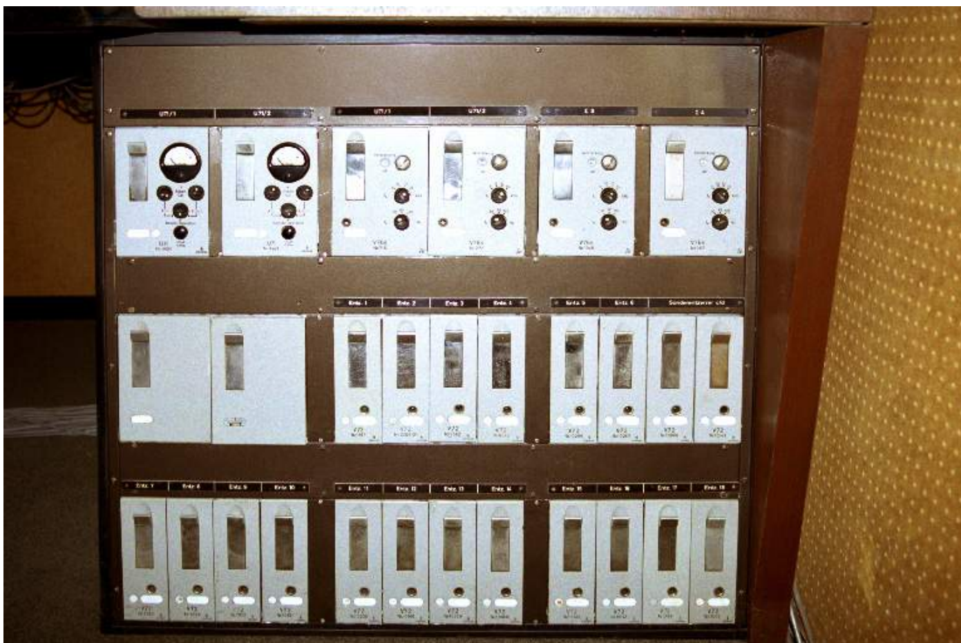
The four output amps are V76`s and the 18 EQ`s are powered by more V72`s.
