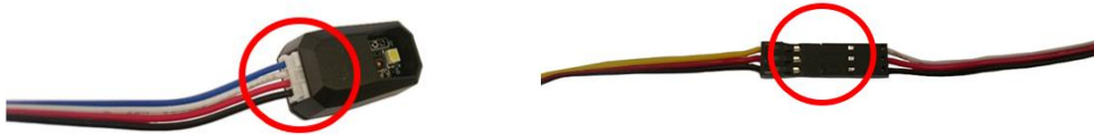
Figure 41 – Electrostatic shocks can occur at poorly insulated or exposed portions of the electronics.
