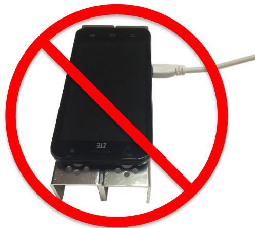
Figure 6: The cable is not supported and is easily damaged or disconnected. The phone is also in direct contact with metal.
