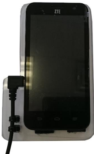
Figure 5: The cable is secured in place. It is still easy to unplug it for charging, but it will be difficult to accidentally unplug. If the phone moves around, there is enough slack to avoid damaging the USB connector
