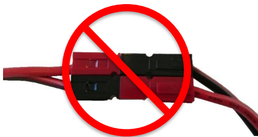
Figure 8: Reversed power wires.
