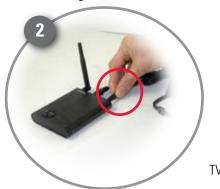
Plug the Receiver power cable into the 9V POWER input. Plug the power adaptor into a wall outlet or surge protector.
