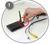
Connect one end of the AV Cable to the back of the receiver. Connect the other end to the Video IN (Yellow) and Audio IN (White) ports on the TV or Monitor for viewing and VCR or DVD Recorder for recording
