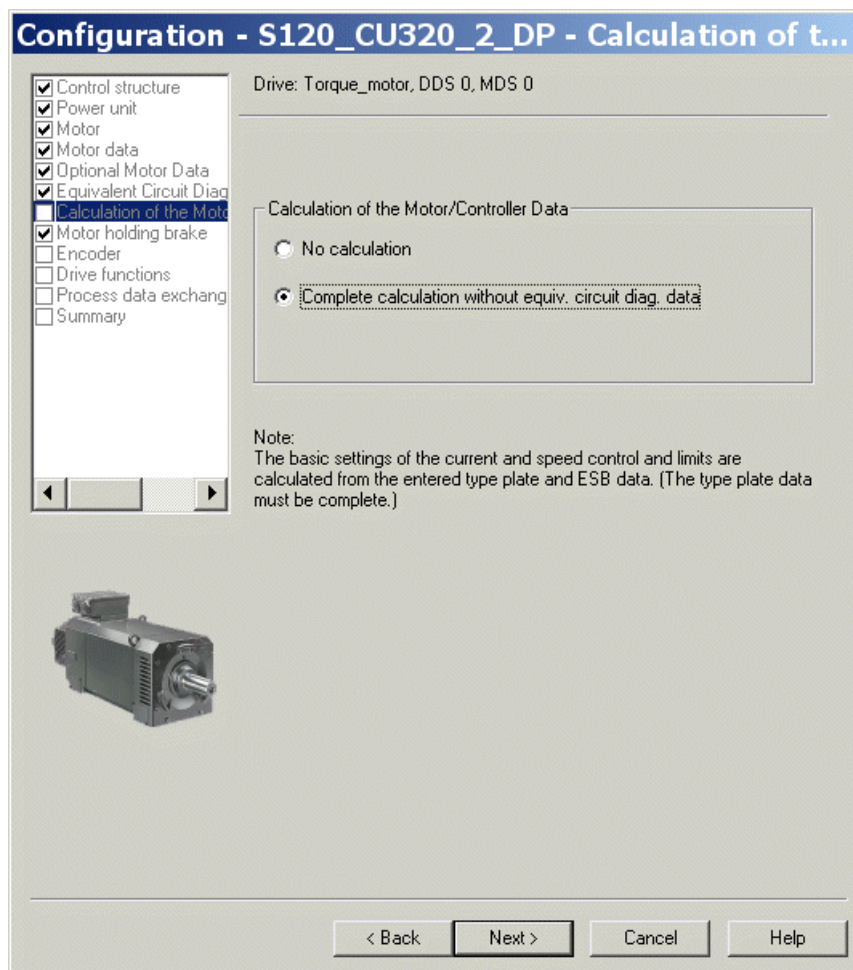
Image 3-76 Screen form for calculating the motor/controller data
