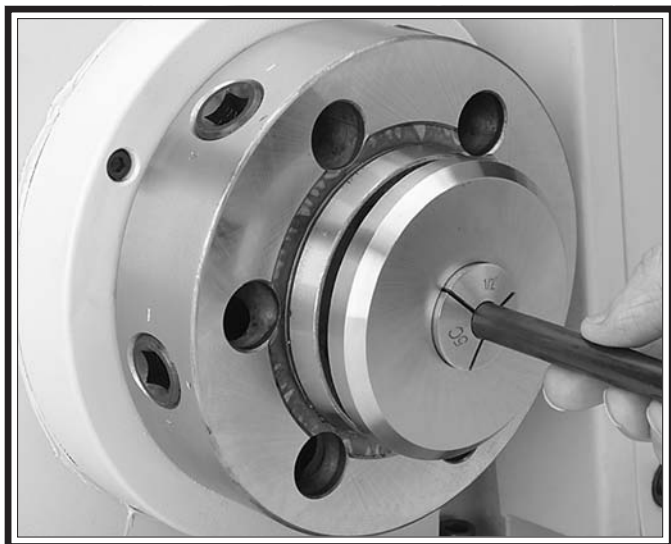
Figure 11. Installing a workpiece.
