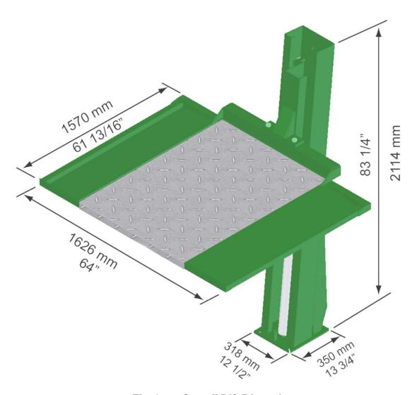
Fig. 1 Overall Lift Dimensions
