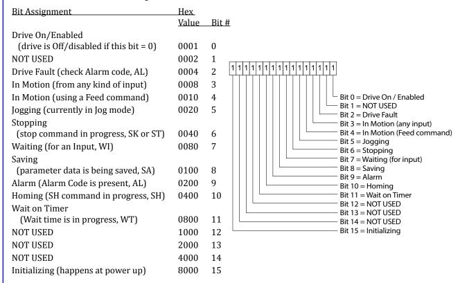
**Example:** The drive is executing an FL command (Bit 4), and it's waiting for the input specified by the WI command (Bit 7). The 16-bit word for this condition is – 0000 0000 1001 0000 – and the hexadecimal equivalent is 90. Therefore, when the host sends "SC", the drive will respond with "SC=90".
