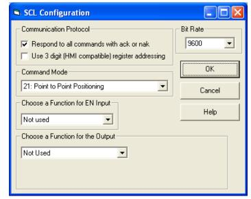
Point-to-point Positioning. See details on the Command Mode (CM) command for more information.
