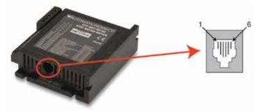
To use SCL in an application means you will have a host device, such as a PC, a PLC, or an HMI, connected to the drive's serial port and using that connection to send commands to the drive. The set of commands defined by SCL includes commands for motion of the step motor, commands for using the three digital inputs, one analog input, and one digital output of the drive, as well as commands for configuring different aspects of the drive like motor current and microstep resolution.
