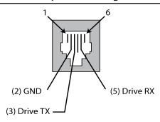
To configure your host to properly communicate with the drive you'll need to configure your host's serial port as follows: 9600 bps, 8 data bits, 1 stop bit, no parity. Not coincidentally, these are the default COM port settings for a Windows-based PC.
