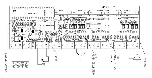
FIGURE 2. SDM-SW8A Address and Port Configuration Jumpers with Sensor Wiring Examples
