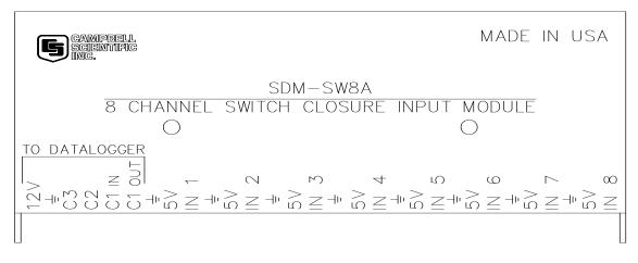
FIGURE 1. SDM-SW8A Front Panel
