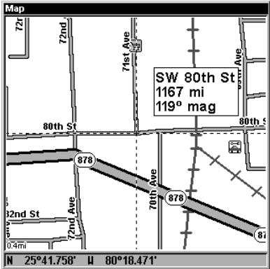
Map Page showing results of an intersection search. The cursor points to the located intersection.
