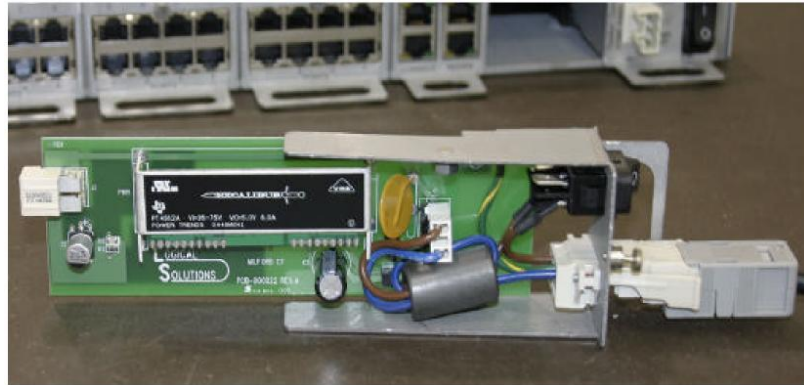
-48VDC Power Module and WAGO Connector (shown removed from Sentinel 32)
