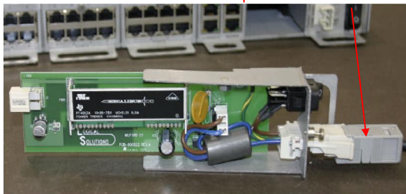
-48VDC Power Supply (removed from back panel)
