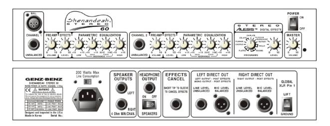
**SPEAKER OUTPUT JACK** – The **Shenandoah™ Stereo 60** provides two ¼" speaker output jacks. Minimum total load is 4 ohms pere side.
