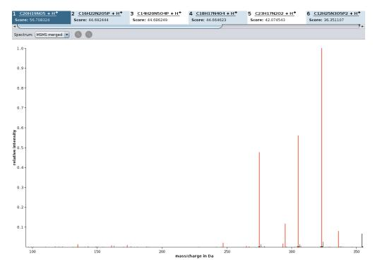
In the *Spectrum view* tab, all peaks that are annotated by the fragmentation tree are colored in orange. Peaks that are annotated as noise are colored black. Hovering with the mouse over a peak shows its detailed annotation.
