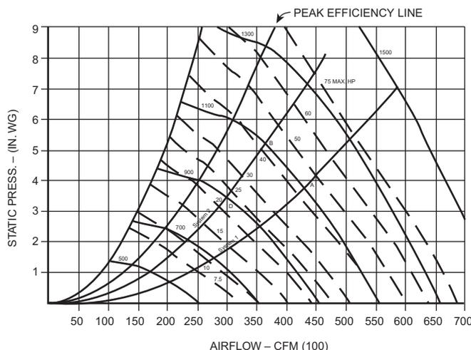
FIG. 3 – FAN CURVE WITH TWO SYSTEM CURVES
