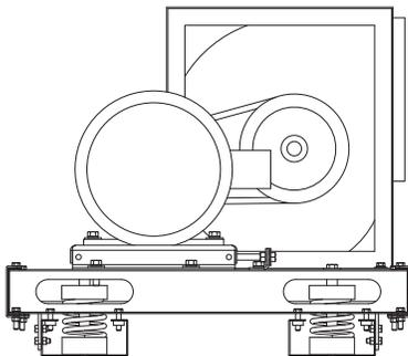
To assure the quietest possible operation, fans and motors are common base isolated from the cabinet.
