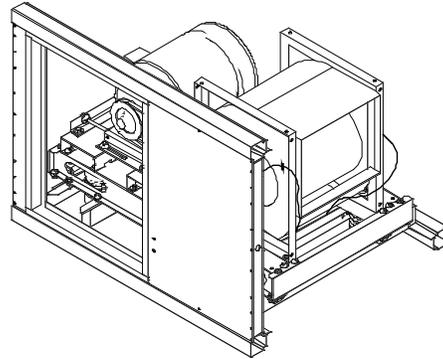
In some situations, there may be a need for a system design using multiple fans in a cabinet. The following are some reasons to consider a dual fan arrangement:
