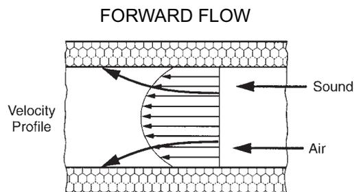
Under FORWARD FLOW conditions, high-frequency sound is refracted into the duct-silencer walls.
