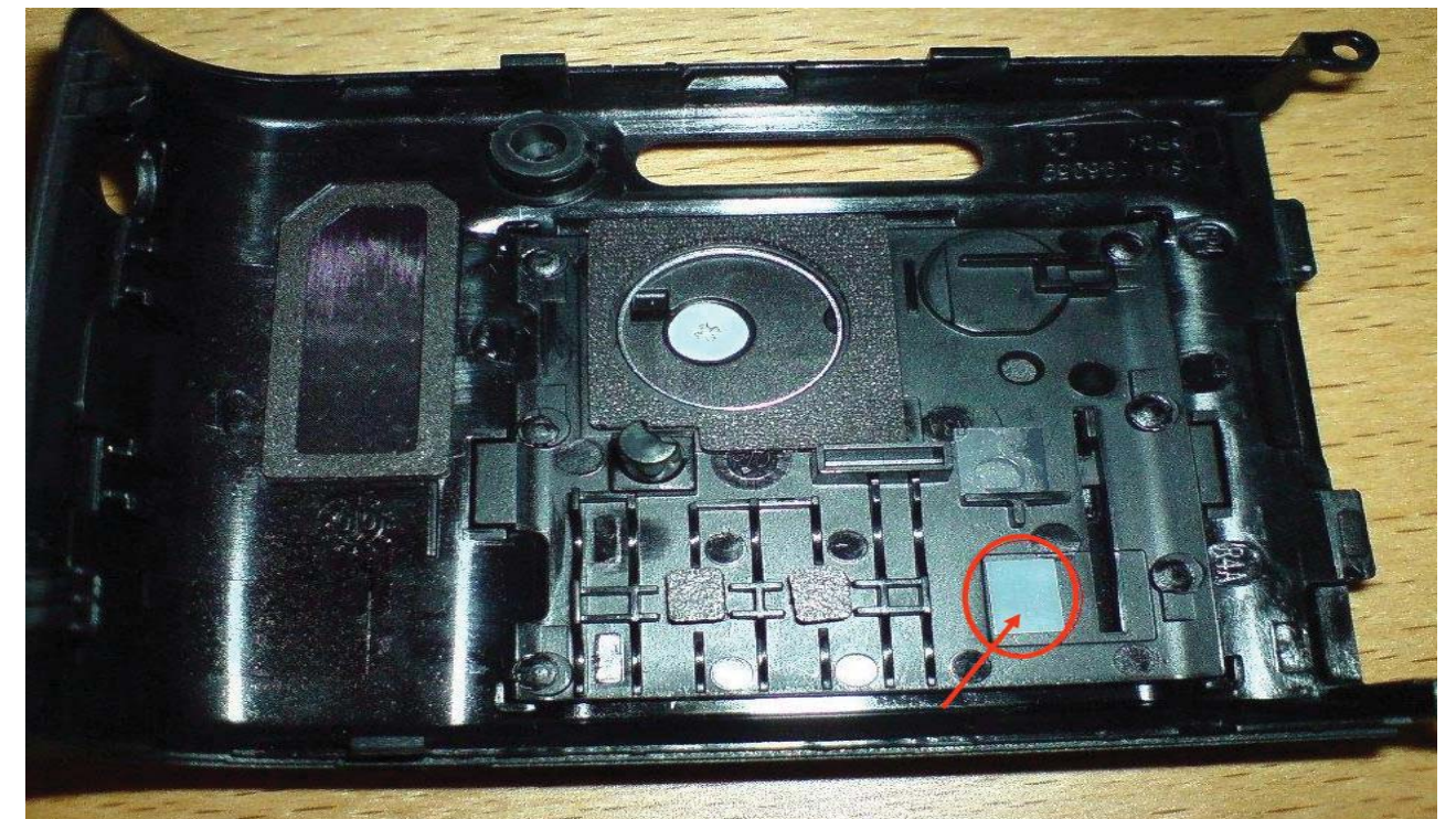
Support pad on the antenna cover.
