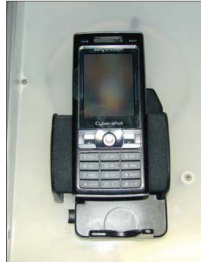
The picture shows how to place the K800-unit in a Rohde & Schwartz Shield Box and Coupler
