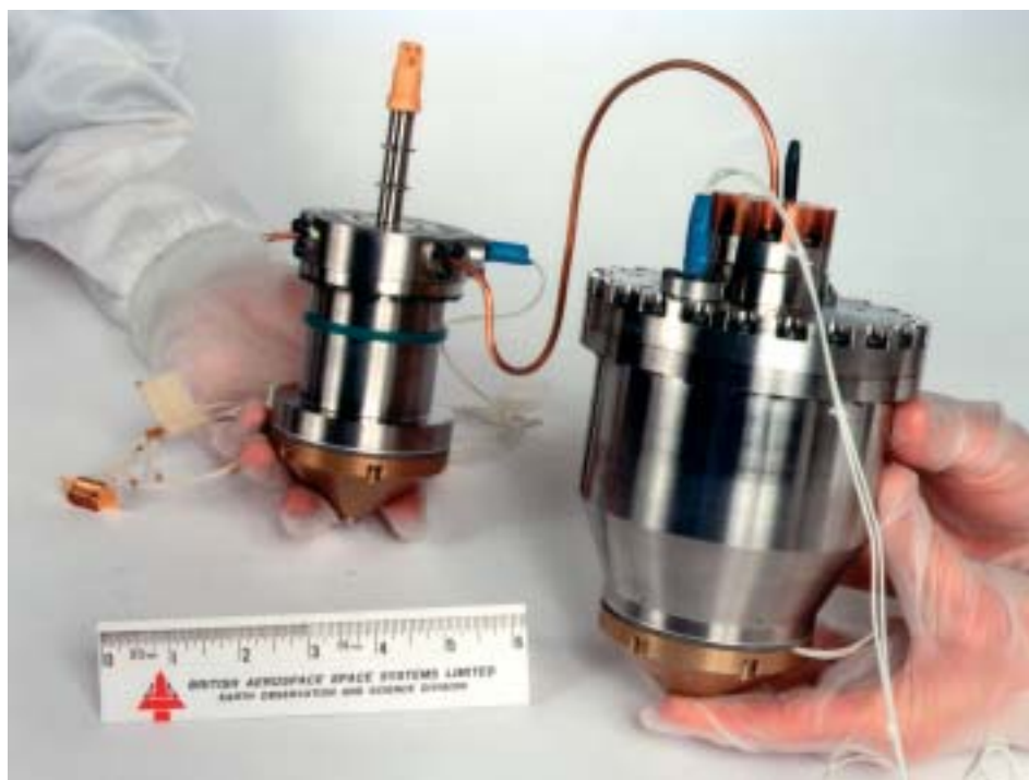
Figure 6.1. The 50-80K Stirling cooler. (Astrium UK)
