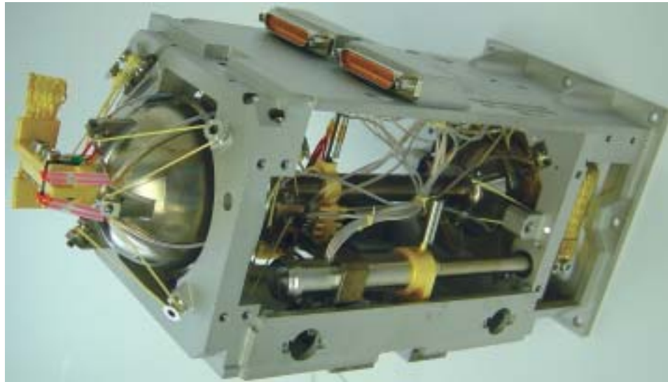
Figure 6.3. Herschel sorption cooler to be used on the SPIRE and PACS instruments.
