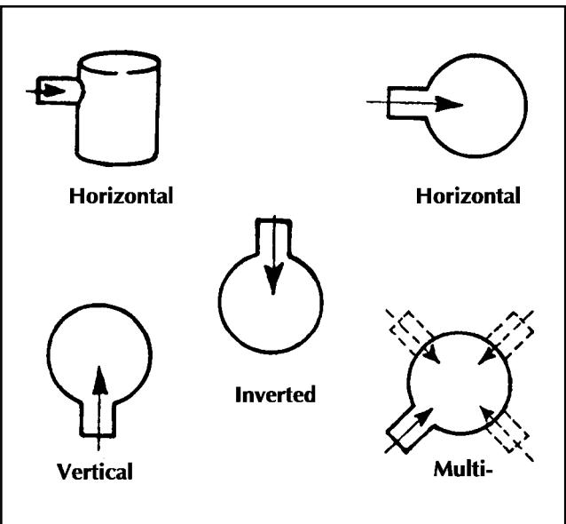
The qualified positions listed include only those tested. In some cases, the manufacturer may claim other positions, but test information at this time neither support or refute such claims. An arrester tilted more than 60 degrees from its qualified operating position may not adequately arrest sparks. Therefore, arresters on mobile equipment—other than screen type arresters—shall not be mounted more than 45 degrees from the qualified position. See column marked "Appl Pos."
