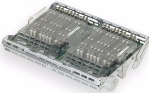
Figure 14. An optional memory mezzanine tray doubles the memory capacity of Oracle's Sun SPARC Enterprise T5240 servers to up to 256 GB.
