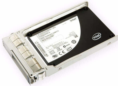
Figure 3. SSDs provide enterprise flash technology in a standard disk drive form factor.
