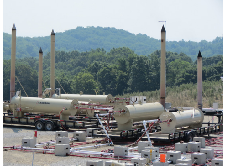
Cameron well test separators feature on-skid piping and instrumentation for simpler maintenance.
