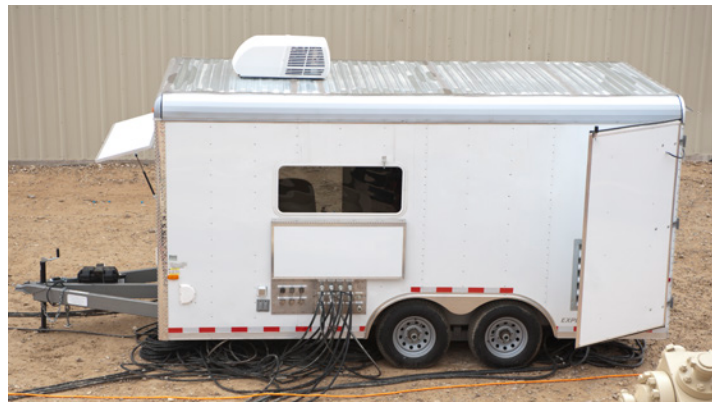
Our hydraulic choke control trailers offer greater functionality for temperature and pressure data acquisition and monitoring.
