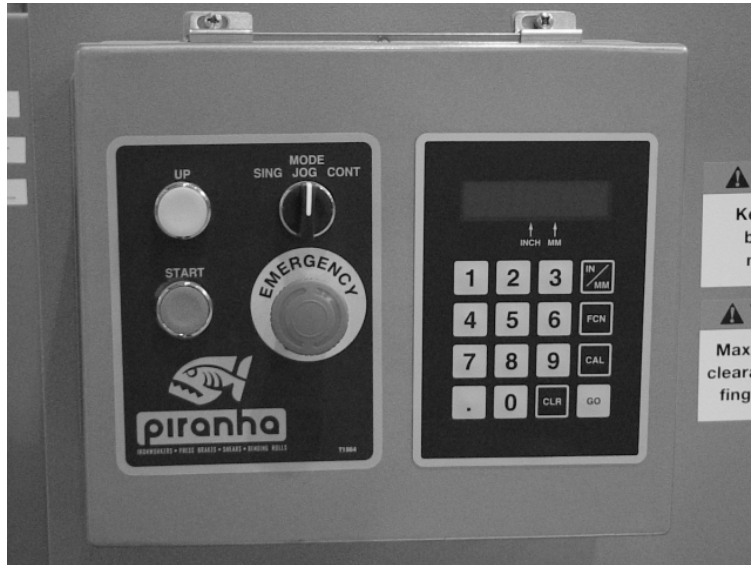
Figure 5: Main Control Panel-Programmable GOTO
