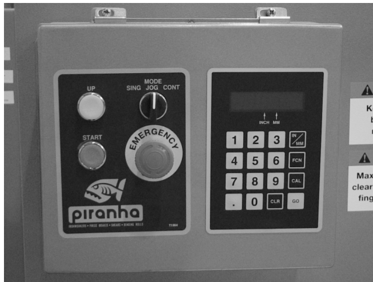
Figure 4: Main Control Panel-Programmable GOTO
