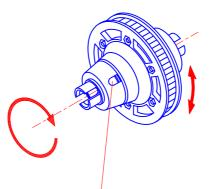
Stick a 1.5mm screwdriver in it that it slots in the head of the diff screw. As you tighten the diff, you will notice the cone washers are being compressed. The cone washers should be tightened until the pulley can not be rotated when both of the diff hubs are being held.
