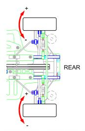
More toe-in will make the car easier to drive out of the corners, but the turn-in of the car will be decreased. Less toe-in will make the car slightly faster and more efficient, but a bad handling car will never make your car faster on the track! Toe-out should never be used in the rear. This can be adjusted on the hingepin adjustment blocks in the center of the the car. Use the rings of 0.4mm for 0.5° settings and 0.8mm for 1° settings.
