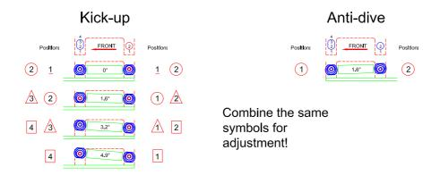
Refers to the angle in which the front suspension is mounted in relation to horizontal when looked from the side of car. Kickup and anti-dive are adjusted by changing the angle of the front wishbones, which can be done by the aluminium hingepin adjustment blocks.
