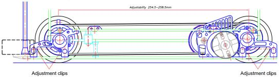
Adjust the wheelbase by moving the black plastic clips.
