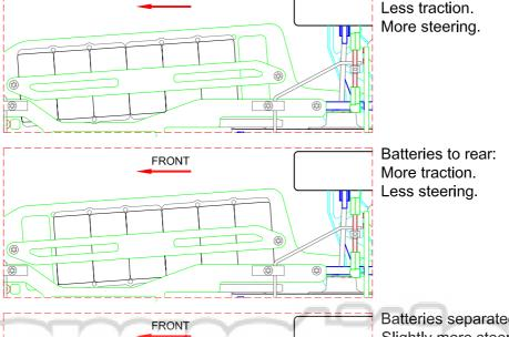
Batteries separated: Slightly more steering. Slightly less rear traction. Easy to drive.
