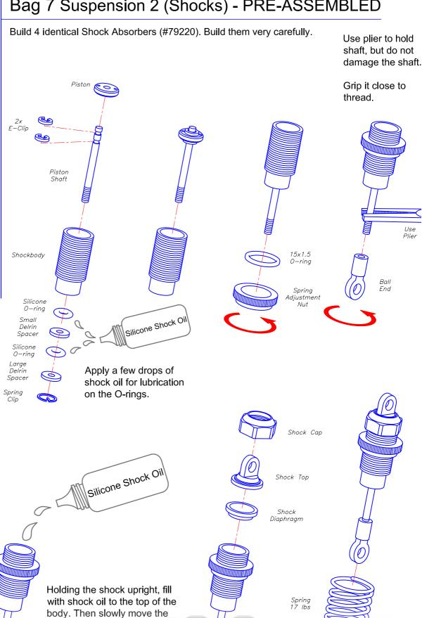
shaft up and down several times to allow air bubbles to escape
