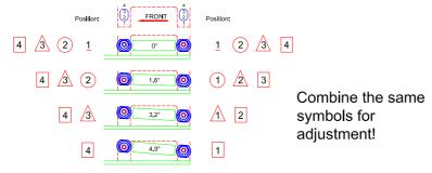
Describes the angle at which the rear supension is mounted when looked at from the side of the car. The setting of 0° anti-squat will give less rear traction, but gives gives more acceleration in bumpy conditions and increase steering slightly. A setup of 1.6° will give some more rear traction, but they will reduce steering. For more rear traction 3.2° and 4.9° are other possibilities, but they will reduce even more steering.
