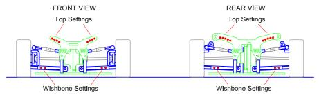
The Assassin allows 4 front and 5 rear top fixing positions for the shock absorbers. The highest setting will make the spring most progressive, which will decrease chassis roll. The lowest setting will make the springs slightly more linear, which will increase grip, but also chassis roll (and therefore decrease cornering speed).
