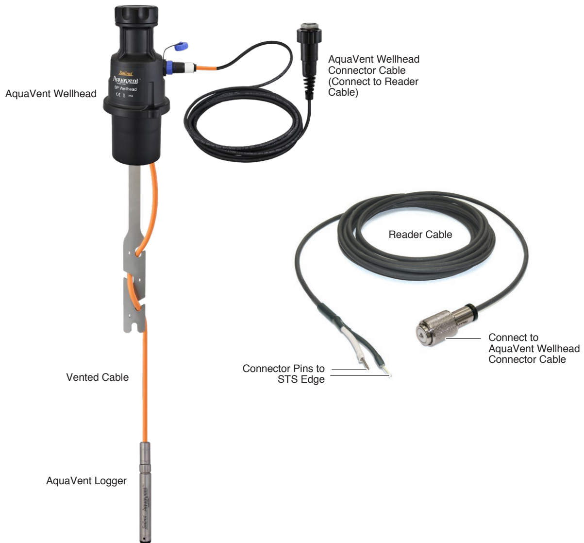
Figure 3-5 Aquavent Connection
