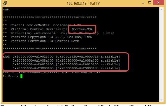
The second line of text shows \*\* Platform: Comtrol DeviceMaster (Cortex-M3) Note the four lines of RAM values shown. This is the NXP Processor.
