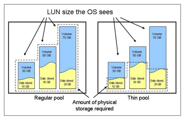
Figure 2 illustrates the advantages of thin provisioning in terms of storage allocation.
