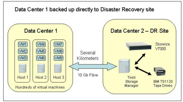
Figure 3 Remote backup solution using Tivoli Storage Manager, Storwize V7000, and TS1120 Tape Drives
