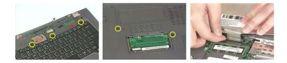
Separate the main unit into the logic upper and the logic lower assembly
