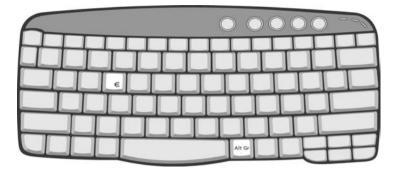
**NOTE:** For US keyboard users: The keyboard layout is set when you first set up Windows. For the Euro symbol to work, the keyboard layout has to be set to United States-International.
