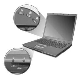
The status LCD displays icons that show the status of the computer and its components.
