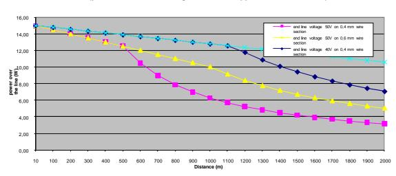
Transmitted power on one pair depending on distance and input voltage (parameter : end line voltage in Volt and copper wire section in mm)
