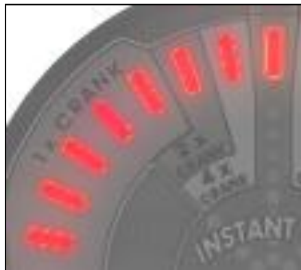
Figure 8. Programming value tach range, 1 to 8
