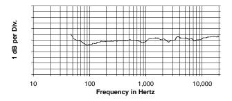
NOTE: The Frequency Response is a plot of the relative difference in acoustic output of a loudspeaker with and without the transformer. Measurement was made at rated output (60W).
