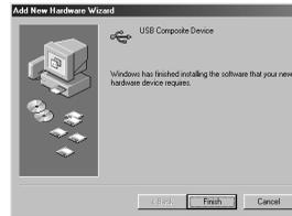
11. Next, the **USB audio device** will be detected automatically, and the **“Add New Hardware Wizard”** dialog box will appear. Click **[Next]**, and proceed with the installation in the same way as in steps **8-11**.
