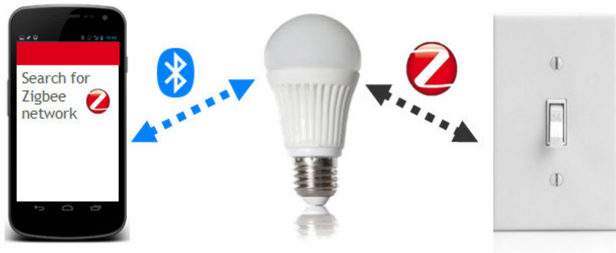
Figure 1.1. Zigbee/Bluetooth Light Example
