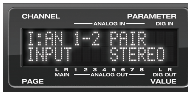
Figure 4-2: The settings for analog inputs 1 and 2 (as a pair).
