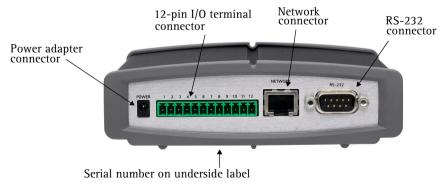
Power adapter connector - Connect the power adapter.
