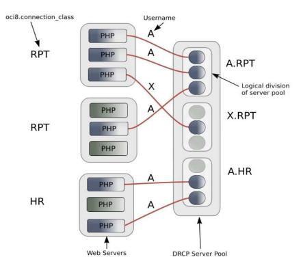
Figure 95: The DRCP pool is logically partitioned by username and connection class.
