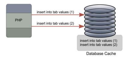
Figure 89: Not binding wastes database resources.
