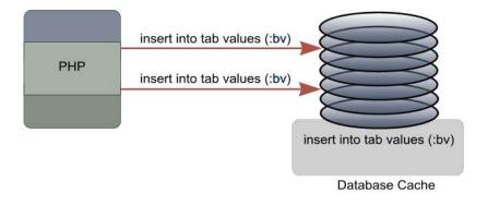
Figure 90: Binding improves performance and security.
