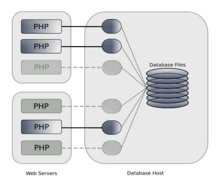
Figure 93: Without DRCP, idle persistent connections from PHP still consume database resources.
