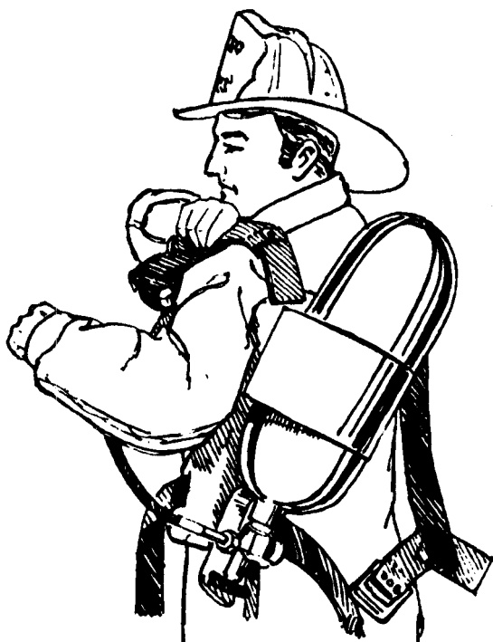
Figure 2-4. Putting on the compressed air, self-contained demand breathing apparatus.
