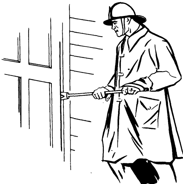
Figure 4-52. Using the door opener.
