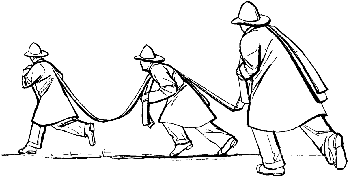
Figure 4-31. Hoving a hose line using shoulder loads.
